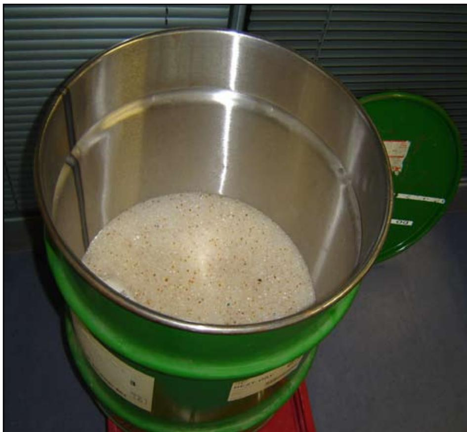
**Figure 13** Silica gel drying bin. (© RBG Kew)
